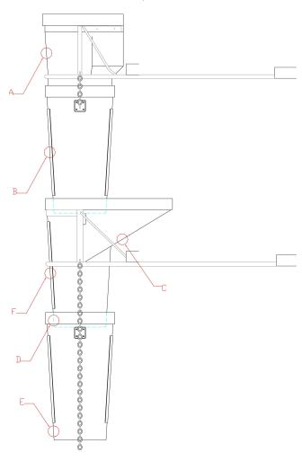
Figure 2 — Impact Points for Falling Mass Test
