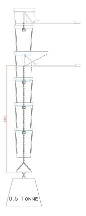
Figure 3 – Test on Support Structure
