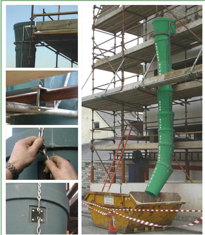
Normally 3 chute section and an Intermediate section are required per floor height
